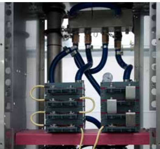
Multiple EV2 units assembled to provide a single 400kW water cooled load
