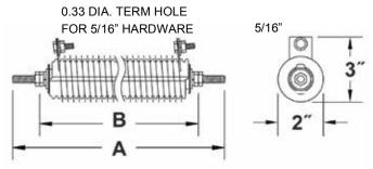
PART NUMBER = EW-SIZE- OHMS X 100 IE: EW5-300 IS RATED 3 OHMS, 18AMPS, SIZE 5
