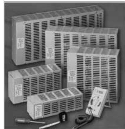
All resistors are factory tested before shipment. This includes a hi-pot test at 2.5 kV for ten seconds on all designs, insuring compatibility for drives systems from 240 to 600V.
