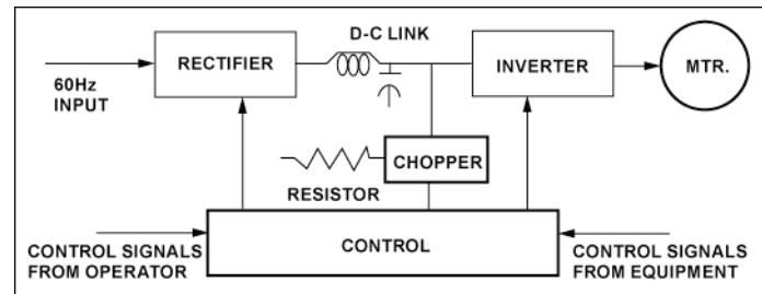
A three-phase variable frequency drive (VFD) consists of three basic components – rectifier, DC line, and inverter – and a control system to manage these three components as illustrated. The rectifier converts the three-phase 60Hz AC input to a DC signal.
